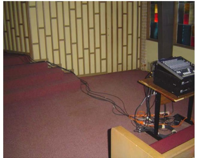
The photo on the left shows a **drainage hole** that should have a protective covering installed. The photo on the right shows **electrical and audio cables** placed on the stairs and walking surface that should be routed away from the walking area, taped to the floor or provided with cord protectors. Areas such as these create unnecessary trip and fall hazards and should be corrected.
